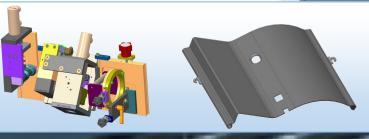
Tool plate for adjusting roll for and hydraulic tool for punching and cutting slat.
